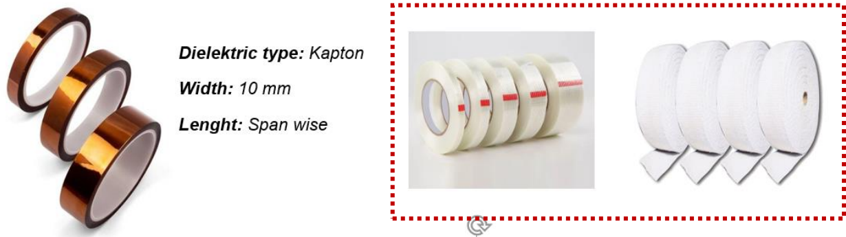
Figure 3. Selected kapton for this project and its specs (left) and other dielectric alternatives fiber glass and ceramic tapes (right)
