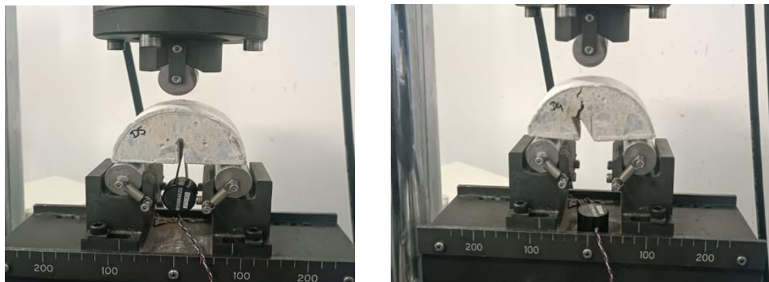
Fig.5 Fracture toughness tests with SCB specimens
